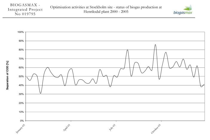
Figure 12. Separation via the pre-sedimentation process during 2003.
