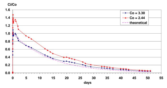
Figure 9. Normalized Li concentration in the effluent from the anaerobic digester 5 as a function of the number of days after dosing of LiCl.
