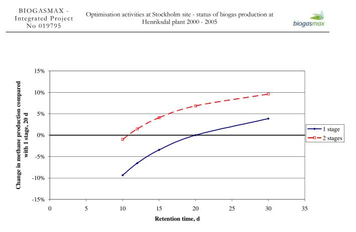
Figure 19. Expected change in methane production in serial operation compared with parallel operation in the case of a retention time of 20 d. Calculations carried out with the aid of data from JTI's digestion investigation corrected with the assumption that degradation takes place approximately twice as quickly in the case of good stirring.
