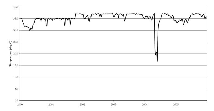
Appendix II – Temperature history in the anaerobic digesters.
