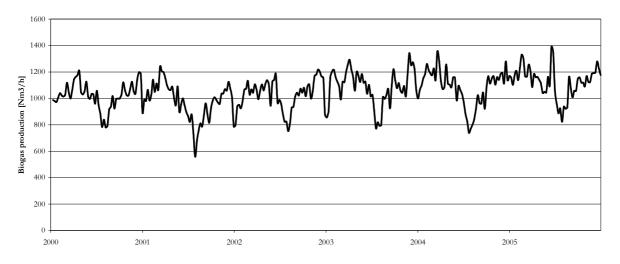
Figure 16. Total biogas flow (Nm<sup>3</sup>/h) from the digestion process during the evaluation period.
