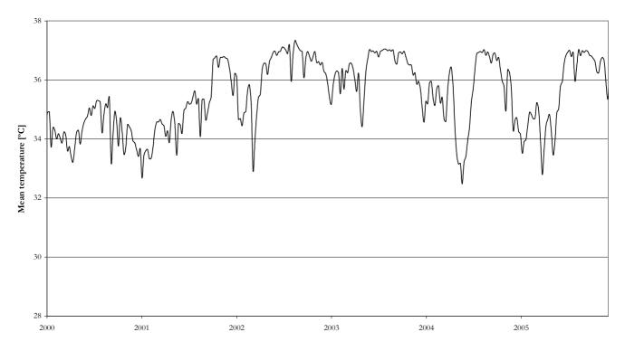
Figure 5. Mean temperature in active anaerobic digesters during the evaluation period.
