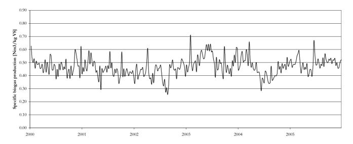
Figure 17. Specific biogas production from the digestion process during the evaluation period.
