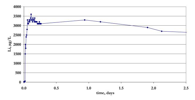
Figure 8. Li concentration in the effluent from the anaerobic digester 5 as a function of the sampling time.
