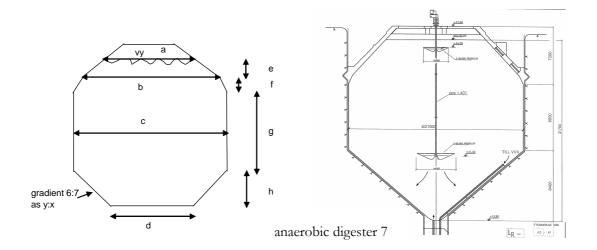
Figure 2. Diagram of an anaerobic digester (not proportional) with dimensions according to Table 2 (on the left), and scale drawing of AD7 (on the right). The top stirrer is not included in this drawing.
