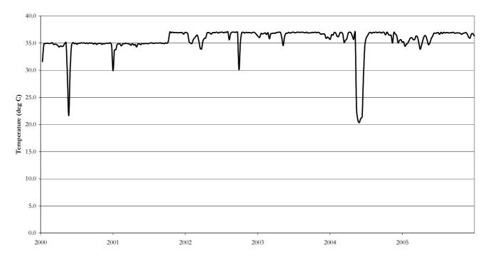
Figure 27. Temperature history for AD2. Values from database henriksdal6m with channel number 164 in WASTE.
