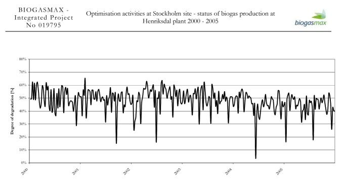
Figure 21. Degree of degradation of the organic matter during the evaluation period, calculated with Formula 8.
