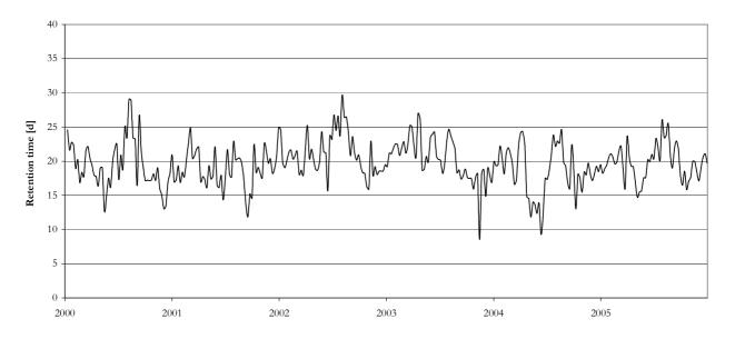
Figure 6. The retention time in the digestion process at Henriksdal calculated from the total volume of all seven anaerobic digesters. Only the volumes of digesters in operation have been considered in the calculation of SRT.
