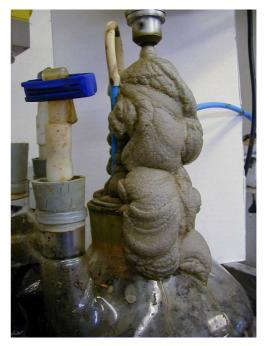
Figure 23. Two experimental reactors from the laboratory at the Tekniska Verken in Linköping for the development of the process aid KMB1. The left-hand photograph shows the experimental reactor with KMB1 added and the right-hand photograph shows the reference reactor. The photographs were taken on the same day; while the experiment was being performed with a high load.
