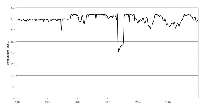
Figure 32. Temperature history for AD7. Values from database henriksdal6m with channel number 169 in WASTE.
