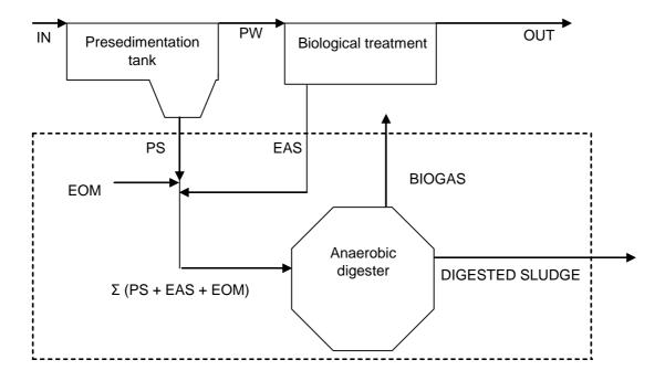
Figure 22. The system limit for COD balance over the digestion process is shown by the dotted line.
