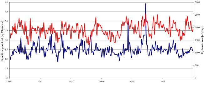
Figure 10. The specific organic load (-----) and the hydraulic load (-----) on the digestion tanks.
