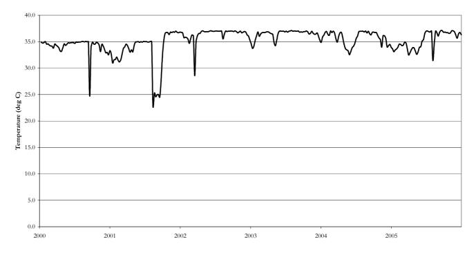
Figure 31. Temperature history for AD6. Values from database henriksdal6m with channel number 168 in WASTE.
