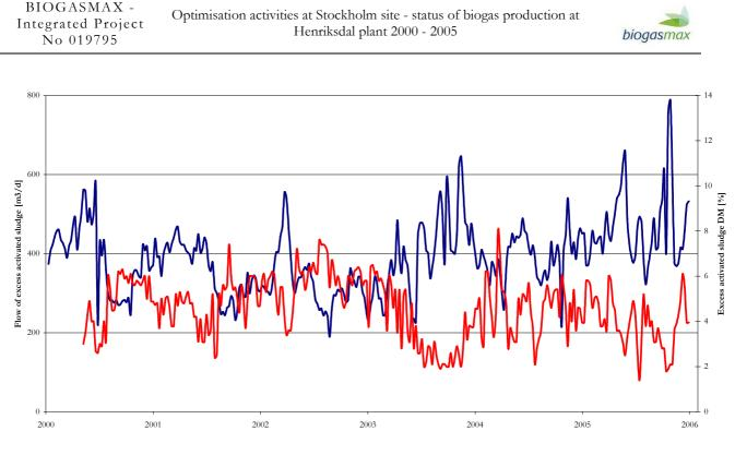
Figure 13. Flow (—) and DM concentration (—) of thickened excess activated sludge pumped to the digestion process.
