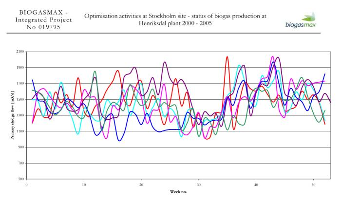
Figure 11. Primary sludge flow for the digestion process during 2000 - 2005 varies with the season. The values are floating means for four weeks so as to identify annual variations more clearly. Years 2000 (--), 2001 (--), 2002 (--), 2003 (--), 2004 (--) and 2005 (--).
