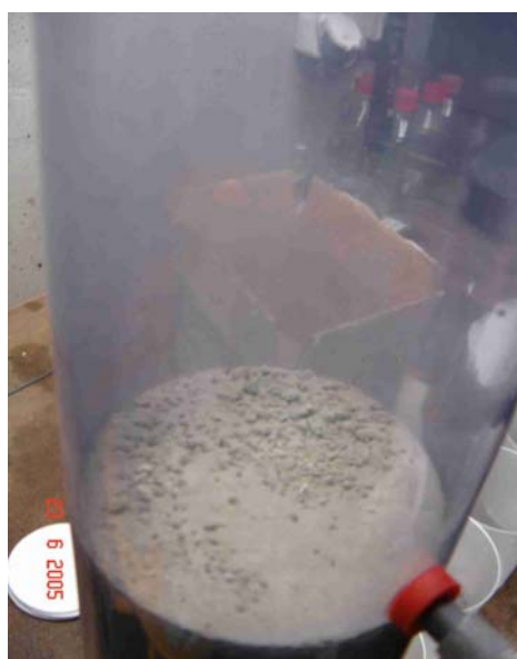
Figure 6. Clogging visible as the effect of outwashing and sedimentation of zeolite very fine particles in the column
